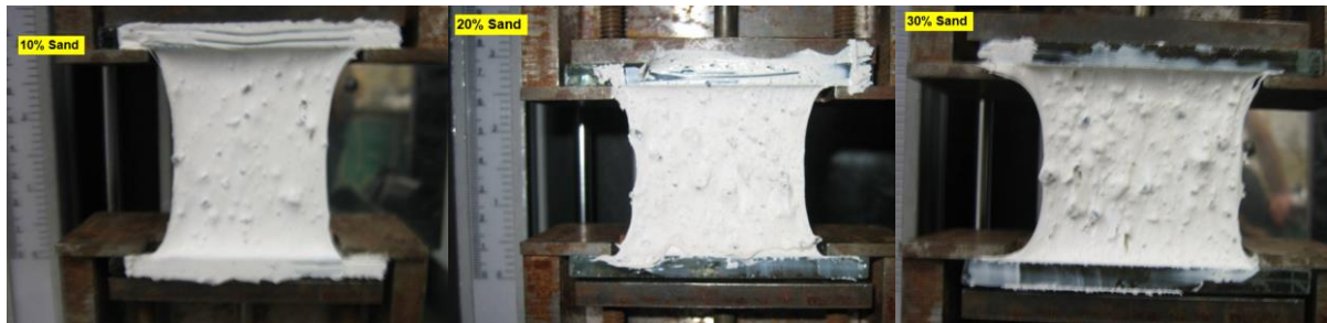
The effect on the elongation capacity of varying levels of granules mixed into the rubber.
