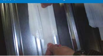
Step 6: Pull polyester fabric at a 90° angle to verify cohesive (pass) or adhesive (potential fail). Picture shows cohesive failure.
